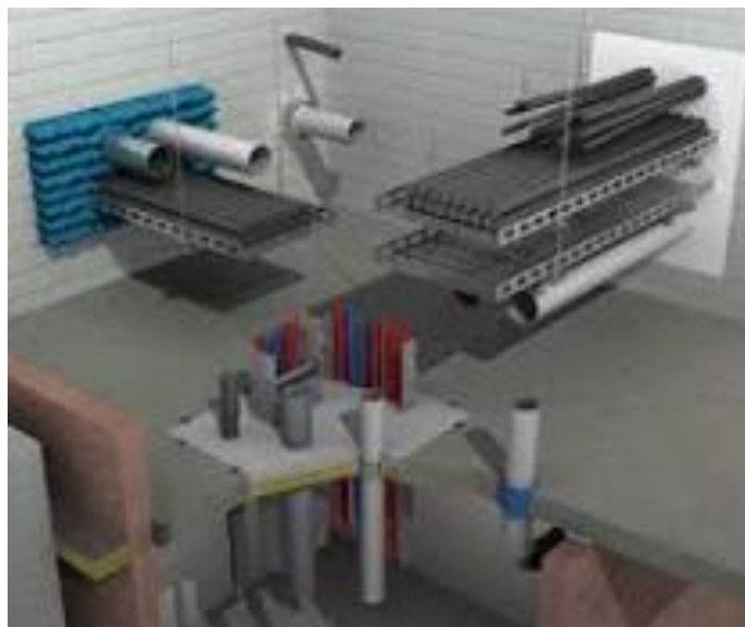
Figure 11 – Example of fire stopping around penetration
