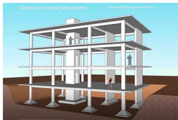
Figure 3 – Precast concrete frame
